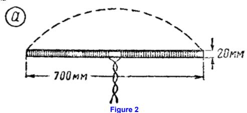
A. Dipole Small Sized Helical Antenna.
