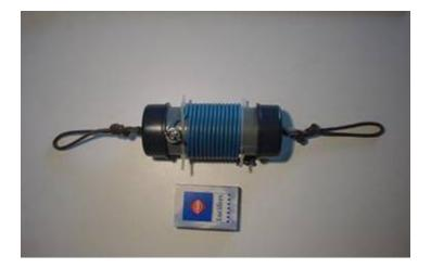
Picture 1: Trap construction with inside capacitor and 5,4  $\mu H$  inductor
