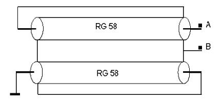
Figure 6. A 1 : 2.25 transmission line transformer.
