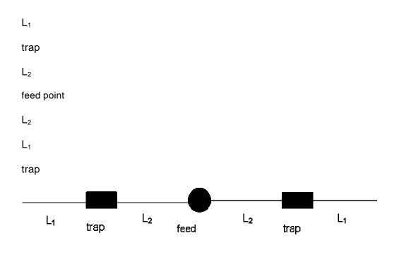
Figure 1: Trap antenna model
