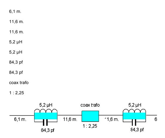
Figure 3: 4-band trap antenna
