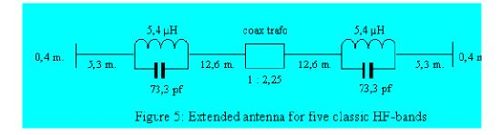
This design will cover all five classical HF amateur bands within SWR < 4 limits. As the design is equal to figure 4 except for the top capacitors, both may be tested using identical components.
