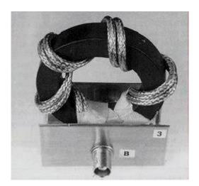
Connection details may be taken from figure 6. Feed line is connected between position B and ground; between position A and ground one will find 1,5 times the input voltage, so 2,25 time impedance.
