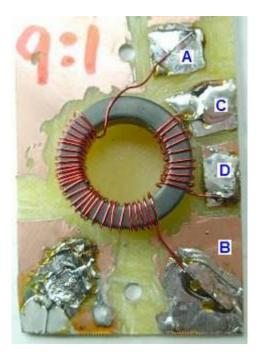
Next I tried a 9:1 impedance ratio UNUN. This an extremely popular impedance transformation ratio for end-fed or random wire SWL antennas. I wound 30 primary and 10 secondary turns on a FT114-43 ferrite torroid. The connection points are identical to those described in the above 4:1 UNUN. Remember that the impedance transformation ratio is the square of the actual turns ratio on your transformer; thus my 3:1 turns ratio is a 9:1 impedance ratio.
