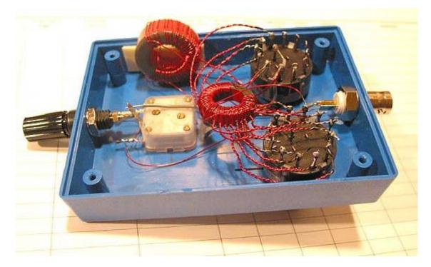
The tuning capacitor is from an old AM radio, and the toroids are a T80-2 and a T106-2 from Amidon.
