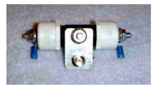
Figure 11: Completed feedpoint insulator
