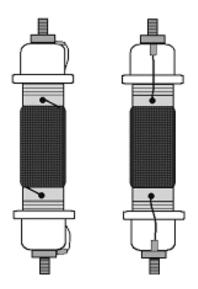
Figure 5: Completed coil
