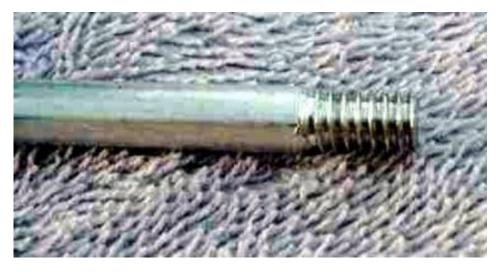
Figure 7B: Completed threads
