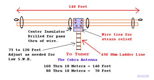
The close spaced wire elements on each leg introduces two added resonant responses BELOW the antenna's fundamental operating frequency.
