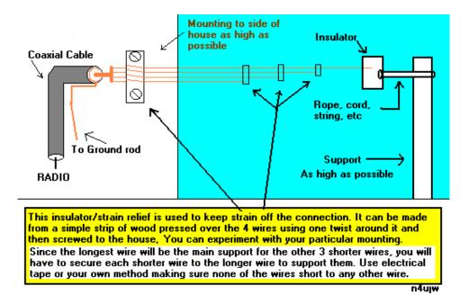
Note: In the instruction box above, the last sentence refers to the long portion of the wires, not at the connection point to the coax feed line to the receiver. All wires are connected together at the connector center conductor wire!
