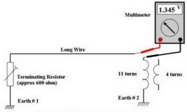
Figure 4: Earth Resistance Measurement
