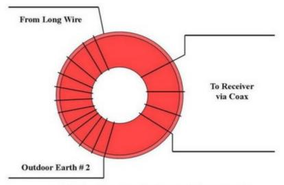
Fig 2: Transformer Winding Detail (12:4 turns shown)
