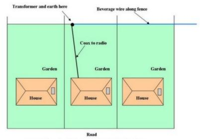
Figure 3: Example of Urban Beverage Installation; Plan View
