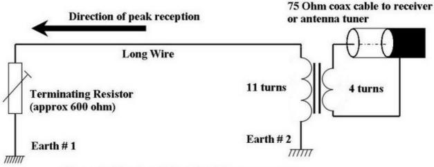
Figure 1: A basic uni-directional Beverage antenna
