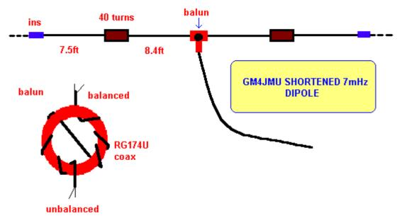
The shortened dipole for 7 mHz was described by Ken GM4JMU in Sprat 74. It is made from insulated wire - Ken used 24/0076. The coils are wound on 40mm ferrite as above, with 40 turns of the same wire on 1.5 ins PVC tube and may be water proofed if required. The balun at the centre is wound with miniature coax (RG174U). Tuning is best done in the clear and the preferred method of adjusting to resonance employed..
