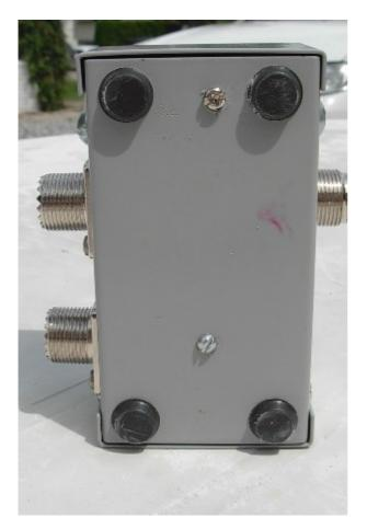
It is really awesome to be able to connect 2 receivers to the same outdoor antenna. The 3 port network and cabling to the additional receiver does not seem to increase receive noise levels from RFI in the house. Most likely this is due to the fact I am using shielded coax, a shielded project box and have a good RF ground system.
