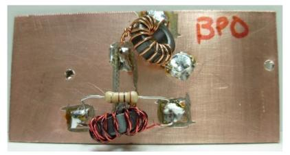
The antenna splitter breadboard is shown to the right. I used 3 colors of 22 gauge enamel covered wire to make my inductors. T2 is the actual splitter network coil and is the lower transformer in the photograph. The 100 ohm resistor serves to isolate the 2 ports connected to the receivers and absorbs impedance mismatches which may present when one terminal is not properly terminated.
