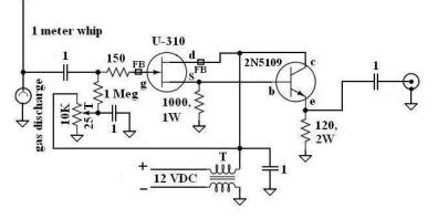
2N5109, so a heat sink is advisable. The U-310 draws about 18 mA, and while it runs quite warm to the touch, a heat sink is not really necessary for it. I used separate 1 mH common mode chokes for T instead of a 2.7 mH bifilar choke. The 24 VDC AC/DC power supply mods were evaluated using an ultra high intercept whip (+50 / +100 dBm II3 / II2) which I have agreed not to disclose.
