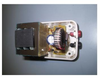
from the outside. On both power supplies I used insulated banana jacks, Radio Shack # 274-725B. The flimsy two wire (white) DC power cords of both power supplies were removed and discarded. The PC board solder pads where the DC power cords were removed were used for the mods. Banana plugs were used to connect the twin lead power feed of the active antennas to the power supplies banana jacks.
