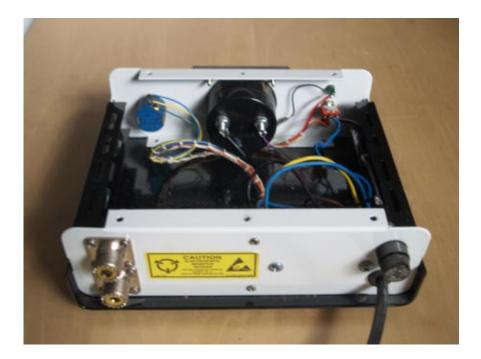
Fig. 9 - Active Antenna Power and Control Unit Prototype Front View (top) and Rear View (bottom)
