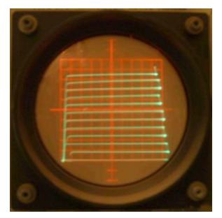
Fig. 4 - 2N2222 Characteristic Curves (horizontal 1V/div, vertical 2mA/div, 10µA/step)
