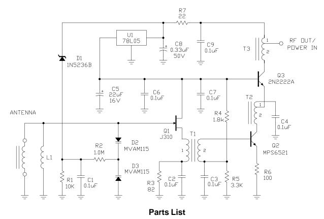
C1, C2, C3, C4, C6, C7, C9 - 0.1uF C5 - 22uF 16V electrolytic C9 - 0.33uF 50V electrolytic
