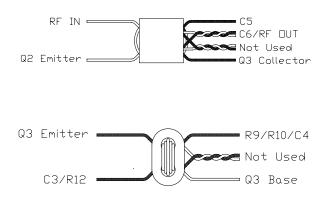
Fig. 8 - Control Unit Transformer Construction Details for T2 (top), and T3 (bottom)
