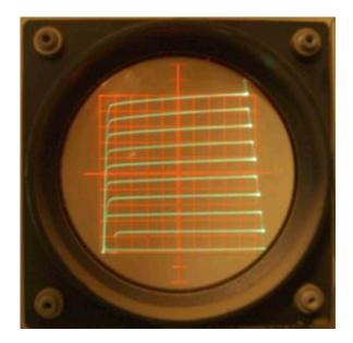
Fig. 3 - MPS6521 Characteristic Curves (horizontal 1V/div, vertical 2mA/div, 5µA/step)
