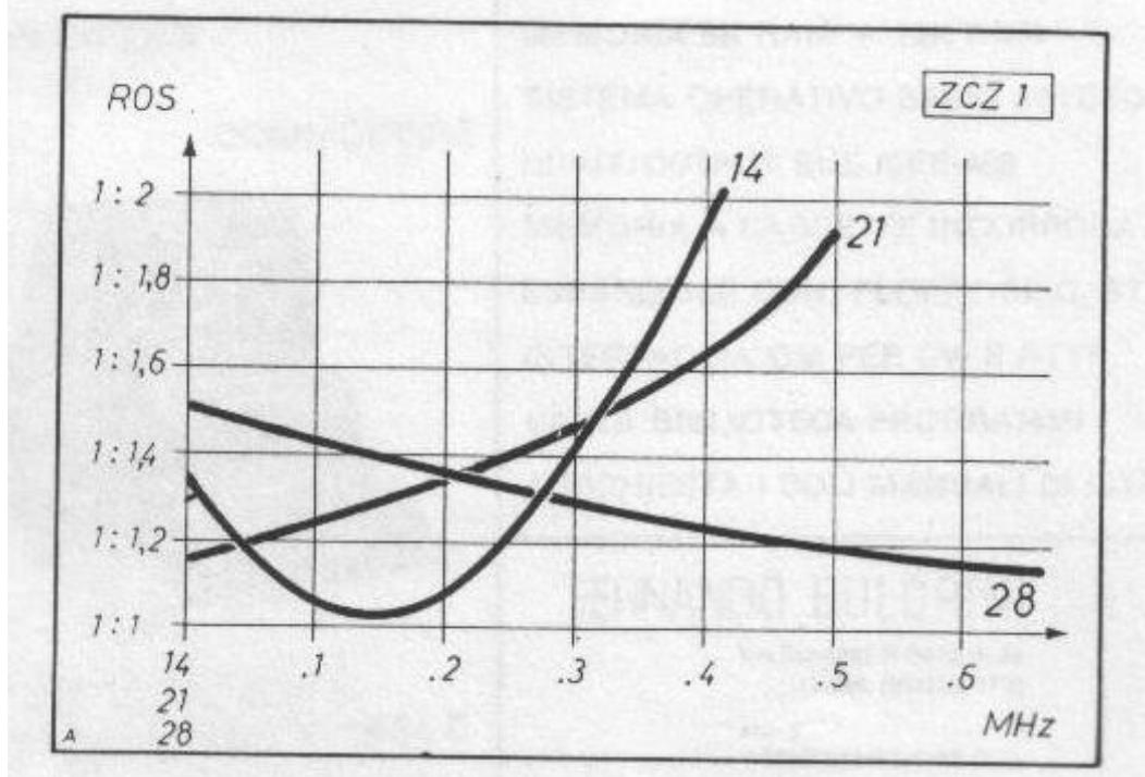
10m = no coil ; 15m = 22 turns (spaced ), 1mm wire diam , coil lenght = 80mm ; 20m = 37 turns same wire and coil lenght.
