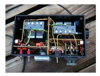
The above picture shows how I mounted the variable capacitors in an opposing configuration. Ideally, the panel knobs would be forward-facing, but the size of the box would not permit such luxury! Nevertheless, I have become used to adjusting the matching unit, and no longer find it tedious to adjust the side-mounted controls for the best match (i.e. minimum meter deflection while in the TUNE position).
