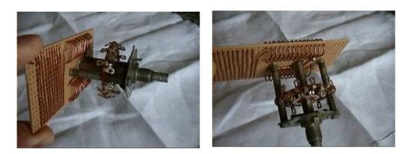
These pictures show the actual contruction of coils A; B; and C after having been mounted on the switch assembly, but prior to wiring.
