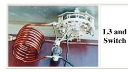
To get over the problem when this occurs, some extra reactance is simply switched in by the addition of L3. In practice, if a match cannot be found by adjustment of Cl and C2, then switch in L3 and try again.
