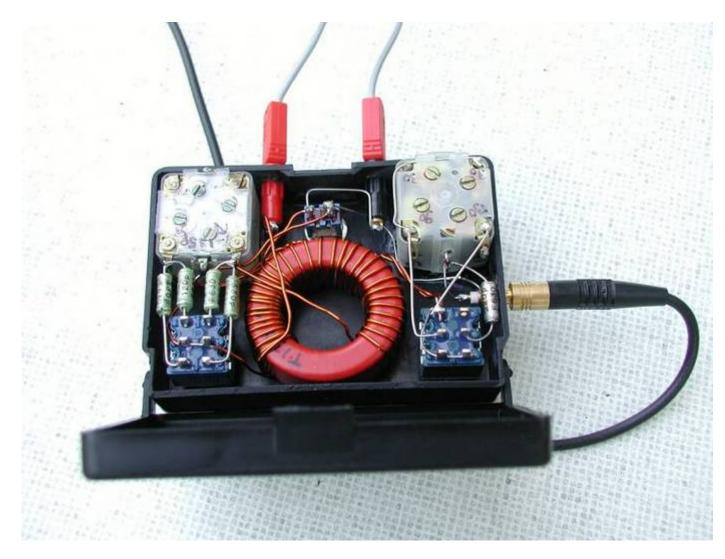
Inside the tuner, the 33mm Amidon core is the largest part. Notice the 630V fixed foil capacitors (four left, one right). Probably you can also use ceramic capacitors, mostly they have lower voltage rating, so try itout. The two antenna connectors are 2mm dia, the 50 ohm connector to the FT817 is an SMB type, coax is 3mm RG174. The 7 turns of the output winding must be wound at the ground part of the primary winding, as indicated in the diagram.
